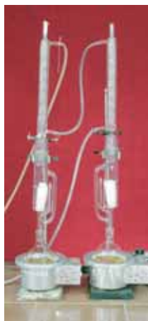
Extraction of oil in Soxhlet apparatus
